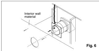
Press the mounting plate tightly against the wall and secure to the outside of the wall sleeve with the supplied screws(screw II). (Fig. 7)
